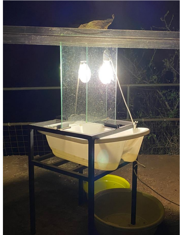
A "modern" light trap with windows and mercury lamp
