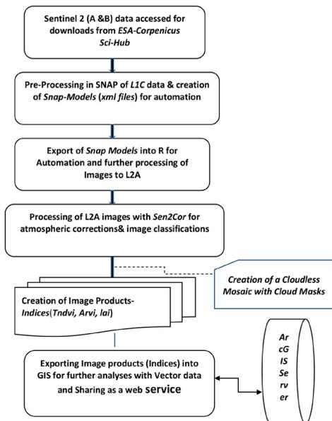
Fig. 2. Workflows for access, processing and sharing Outputs of Image Data from Sentinel-2 through the Tanzania National Parks (TANAPA) GIS Server
